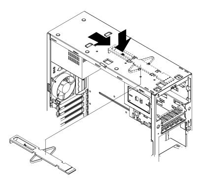
To remove the bezel release latch, do the following:
